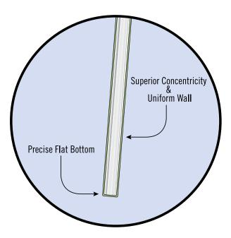
Through our advanced manufacturing process, the NMR tube bottoms are uniformly hemispherical and consistent, thereby minimizing shimming and susceptibility differences among samples. This uniformity extends throughout the wall thickness of the tubes, maximizing the concentricity among tubes and lots. This translates to more consistent placement of the contained sample volumes in today's advanced, highly homogeneous, high field NMR magnets.
