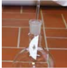
How it should be: The blade has an excentric bore. It tilts and can easily be removed from the vessel.
