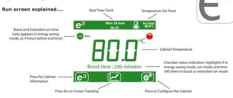
The control system on the E3 Cabinet is designed to be energy efficient. The cabinets will turn warm up in-between the hours of 7am and 7pm Monday to Friday only. The operator can perform a boost start before 7am (or at weekends) or an extended run time after 7pm, however, the cabinet will then reset to default times. If you want to change the default time settings, contact the manufacturer for the password.
