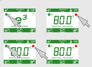
The cabinet will always be in run mode between the hours of 7am and 7pm Monday to Friday. If you don't want to warm the cabinet between these hours, either turn off the unit with the on/off master switch or configure the set point to '0' Boost start......
