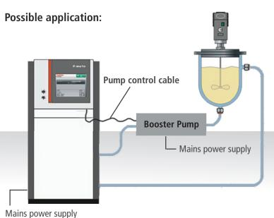
The Mag Drive Booster Pump can increase your fluid pressure up to 2.1 bar. The stainless steel design of the Pump provides excellent resistivity against chemical effects. The magnetically driven design guarantees 100% leakage free operation over an extraordinary temperature range of -90 ... +250°C.
